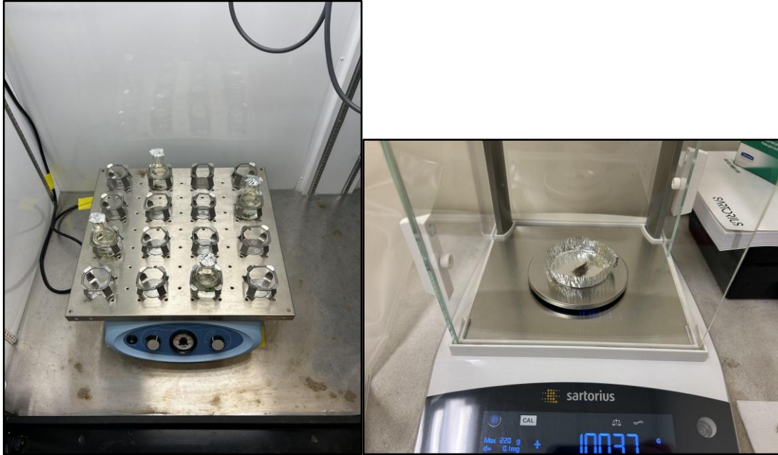
Figure 1. (left) Shaker table holding 4 flasks containing Pithophora samples in unamended river water. (right) Dried Pithophora sample on a weigh boat inside a microbalance.
