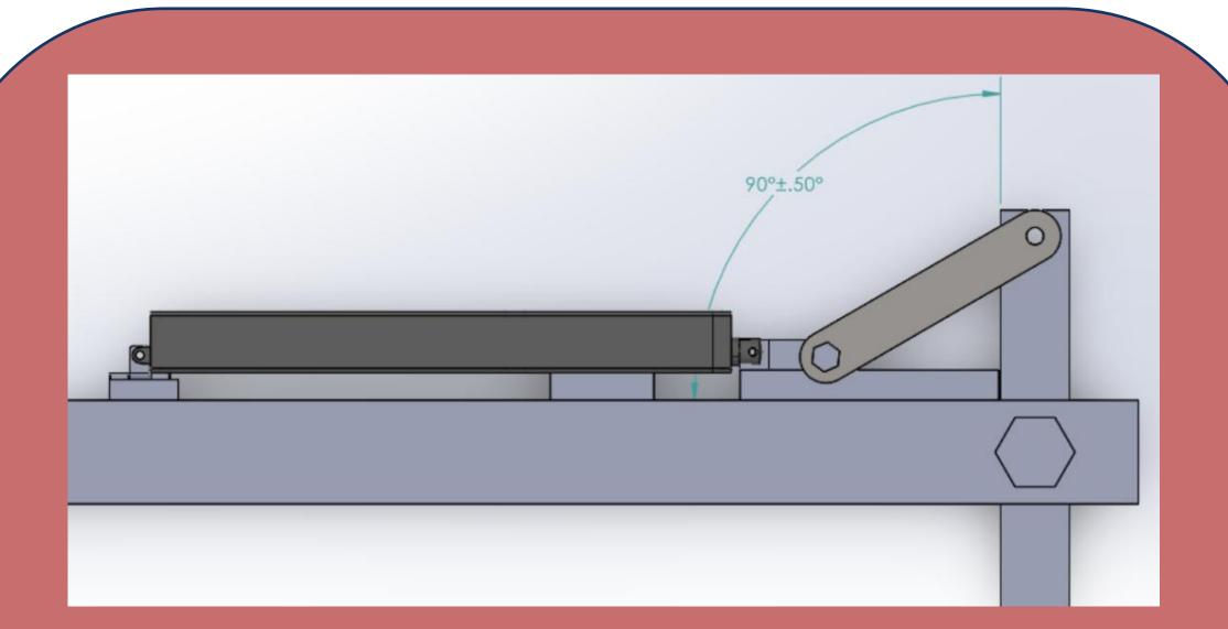
The arm rotates using a 6-inch linear actuator and a 7.5-inch aluminum slide. This setup allows the arm to move between 90° and 150°. Two coupler links connect the slide to the arm, which is held in place with a 1-inch bolt. A thrust bearing at the joint ensures smooth motion without metal parts grinding together.
