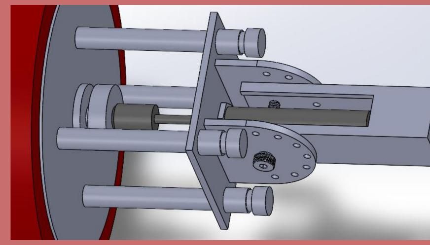
The damping system reduces impact force to protect the machine and user. A foam-padded circular target absorbs kicks and is connected to a shock absorber that compresses to reduce impact energy. Guide rods keep the motion straight and stable.
