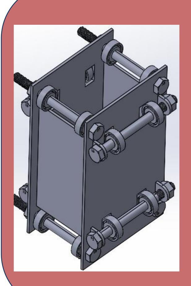
A rectangular trolley moves vertically using a power screw and roller bearings for smooth, stable motion. A fixed support system prevents bending, with bearings spaced by washers and secured with a ½-inch brass rod.
