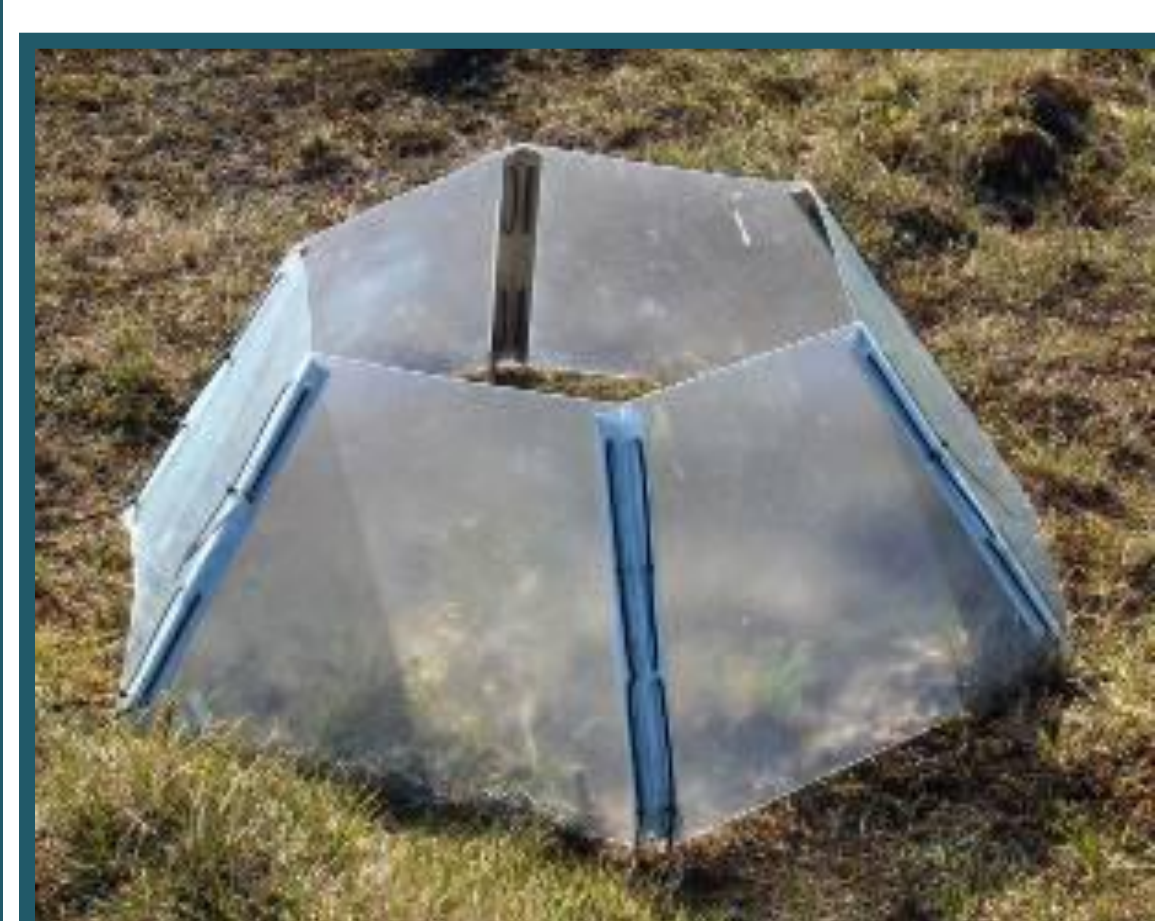
Figure 2 (Below): Open-top chamber used to warm experimental plots
