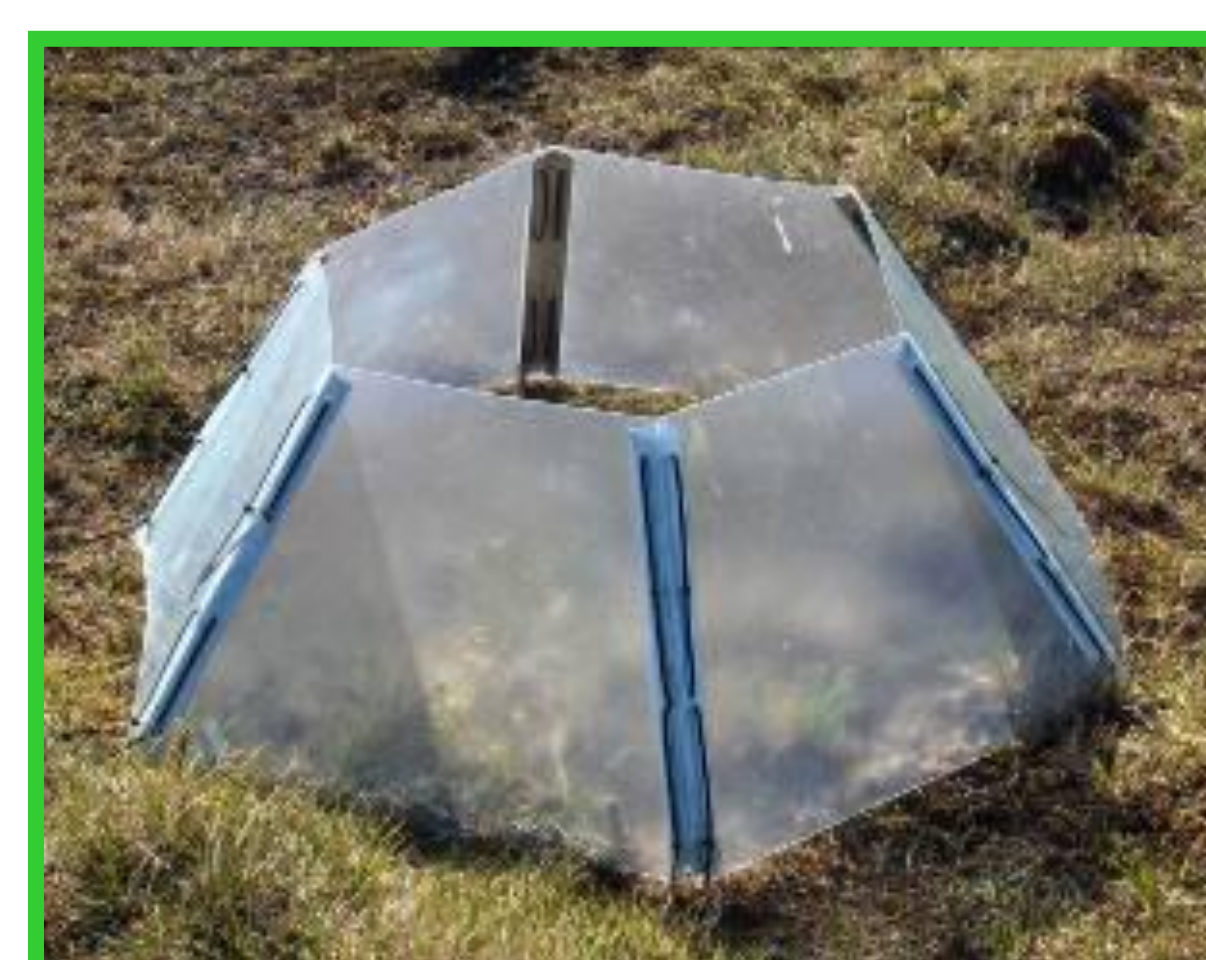
Figure 3 (Below): Open-top chamber used to warm experimental plots
