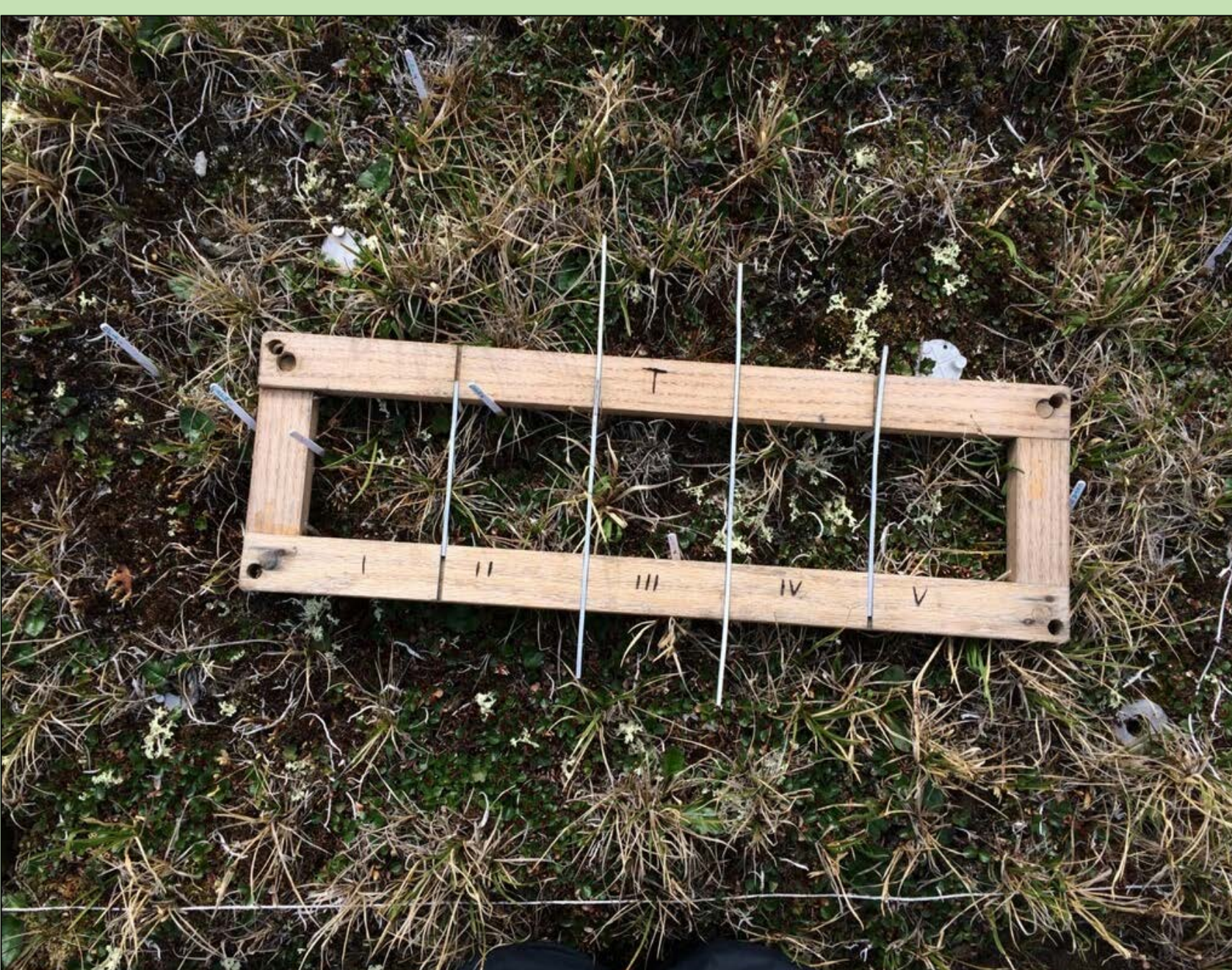
FIG 1. The 10cm by 50cm sampling plot is divided into five 10 cm 2 subplots to measure species density.
