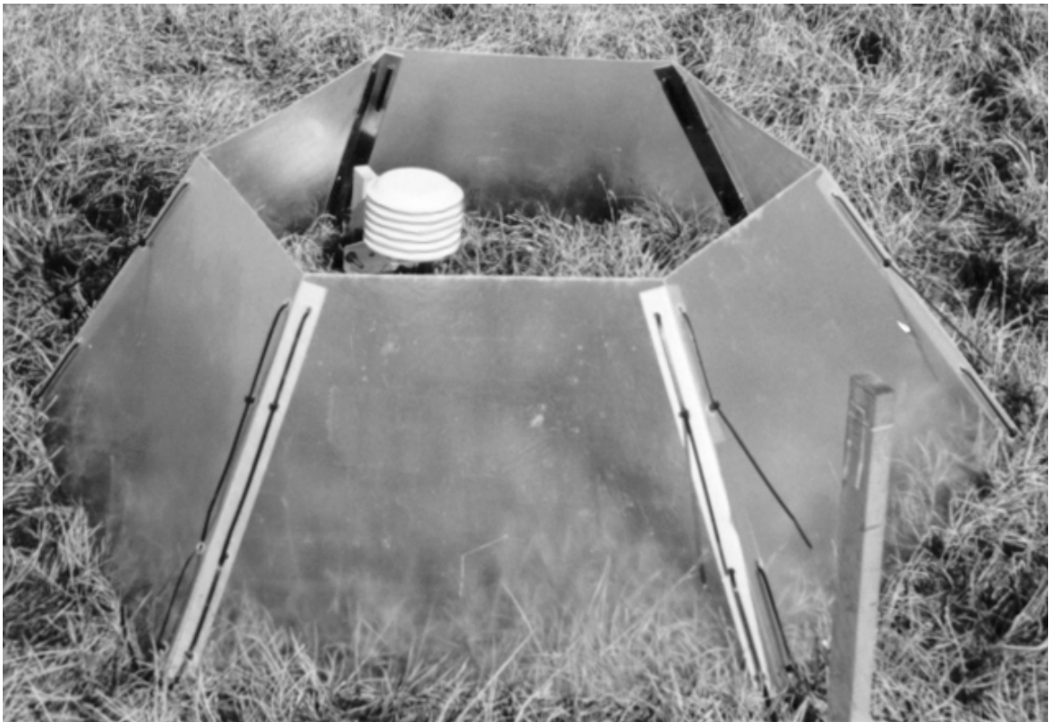
Figure I-5. An open-top chamber (OTC).
