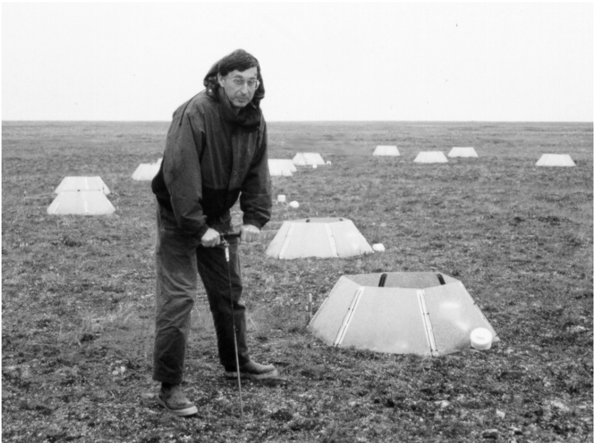
Figure II-9. Probing the active layer.
