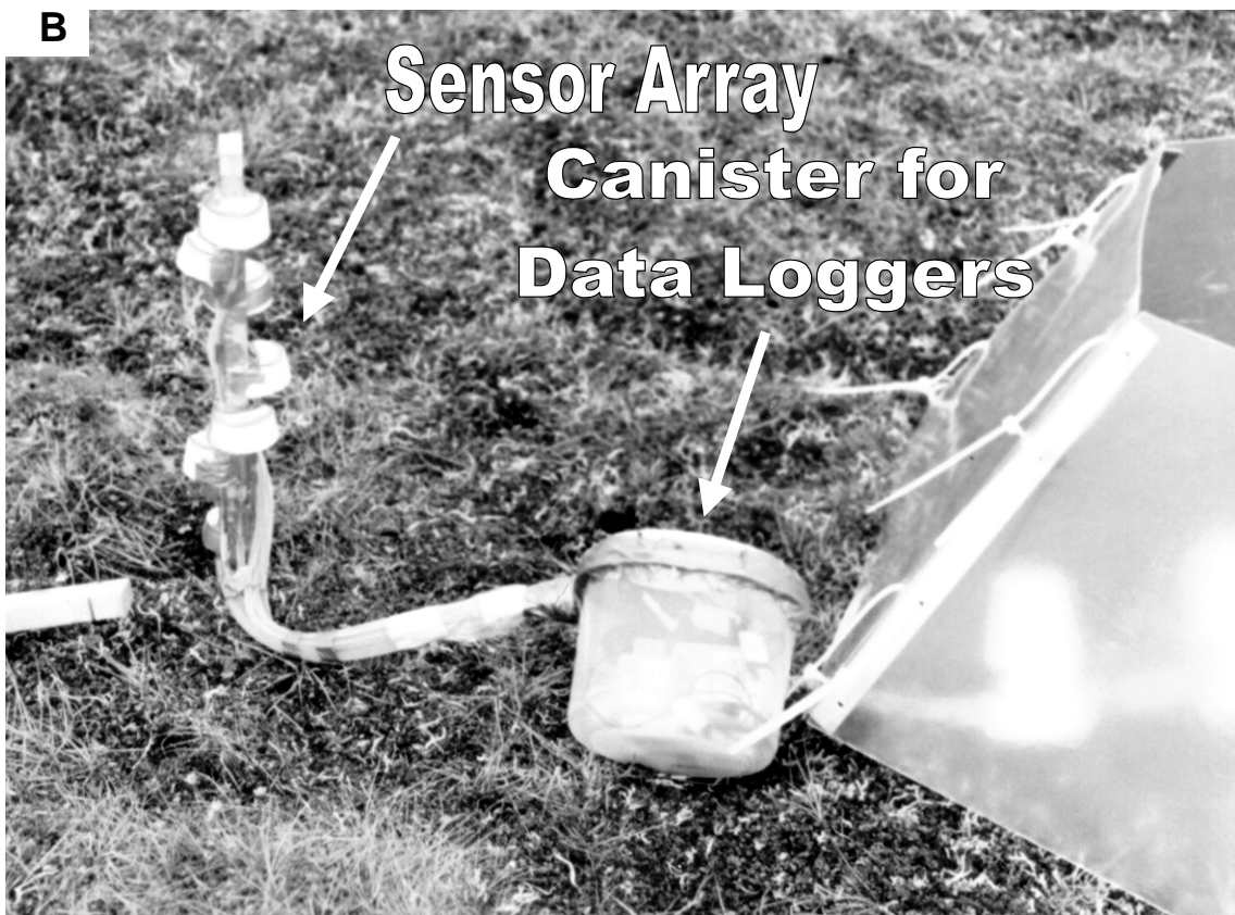
Figure II-6. The spatial arrangement of temperature probes: (A) horizontal distribution and (B) vertical distribution.
