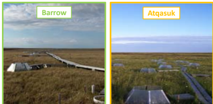
Figure 2. Open top chambers passively warm experimental plots 1-3°C
