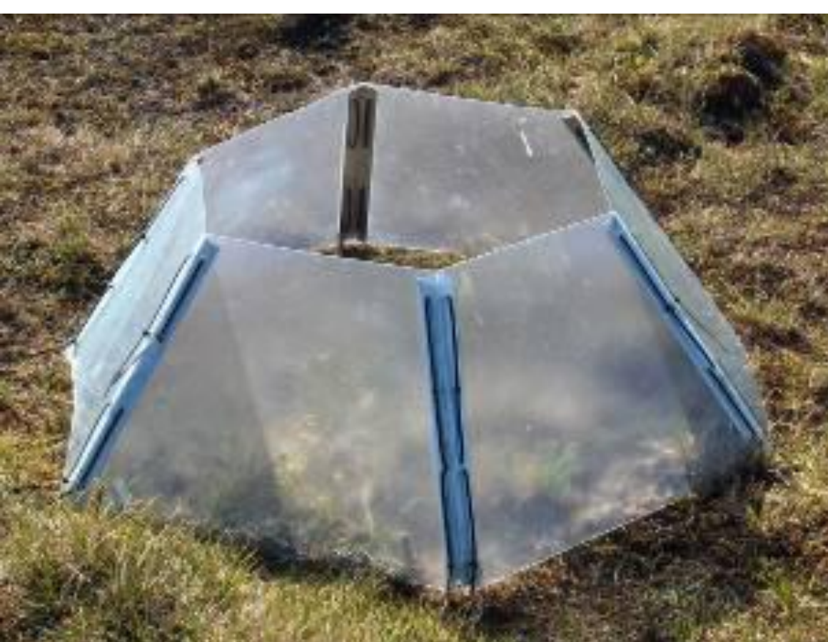
Figure 3: Fiberglass open top chamber used to warm experimental plots.
