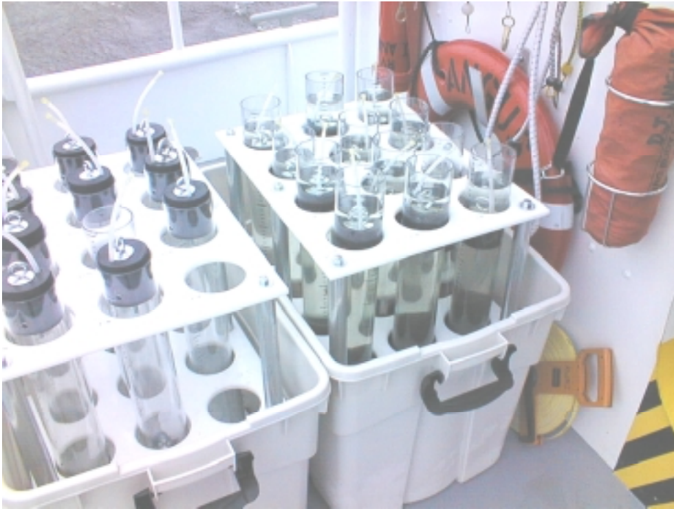
Fig. 2.1.2. Photograph of stoppered tubes (tubes on right with collected cores) seated in holding racks, which are placed in tubs to maintain ambient temperature.
