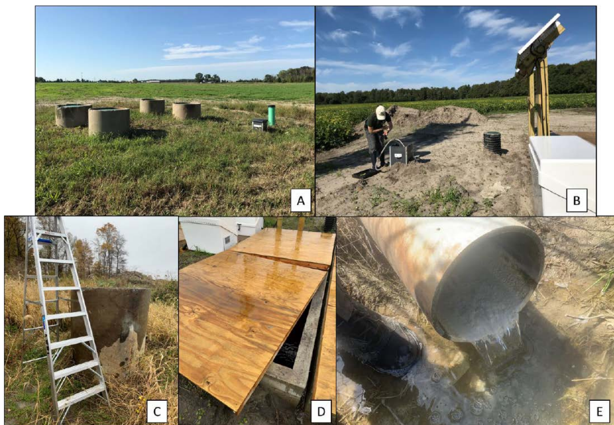
Figure 4. Photos of different sampling locations. A) Behind Mill 1 with completed iron slag filters in place. The green tube (far right) is an inflow sampling port that was installed only at this location. Access ports (for cement upright tubes) are for two slag filter basins (considered to be one slag filter site) that receive tile drain water from the adjoining field (in background) and are used to sample outflow. B) Research Assistant, Emily Kindervater, using a hand pump siphon to sample from a below-ground control box (inflow) at Fillmore Flex; Oak Grove 2 has a similar constructed inflow access (not shown). C) Slag filter outflow access point for Oak Grove 2, which required a ladder to remove the large plastic cap to sample outflow water. D) Slag filter outflow access point at Fillmore Flex, which is covered with large plywood lids. E) Outflow pipe at Behind Mill 1 directly after installation; the white particulate residue inside the tube is from the calcium carbonate layer placed on top of the iron slag inside the tanks to balance pH.
