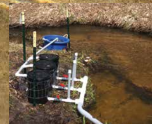
Egg incubators (black buckets) tested in a Manistee River tributary.
