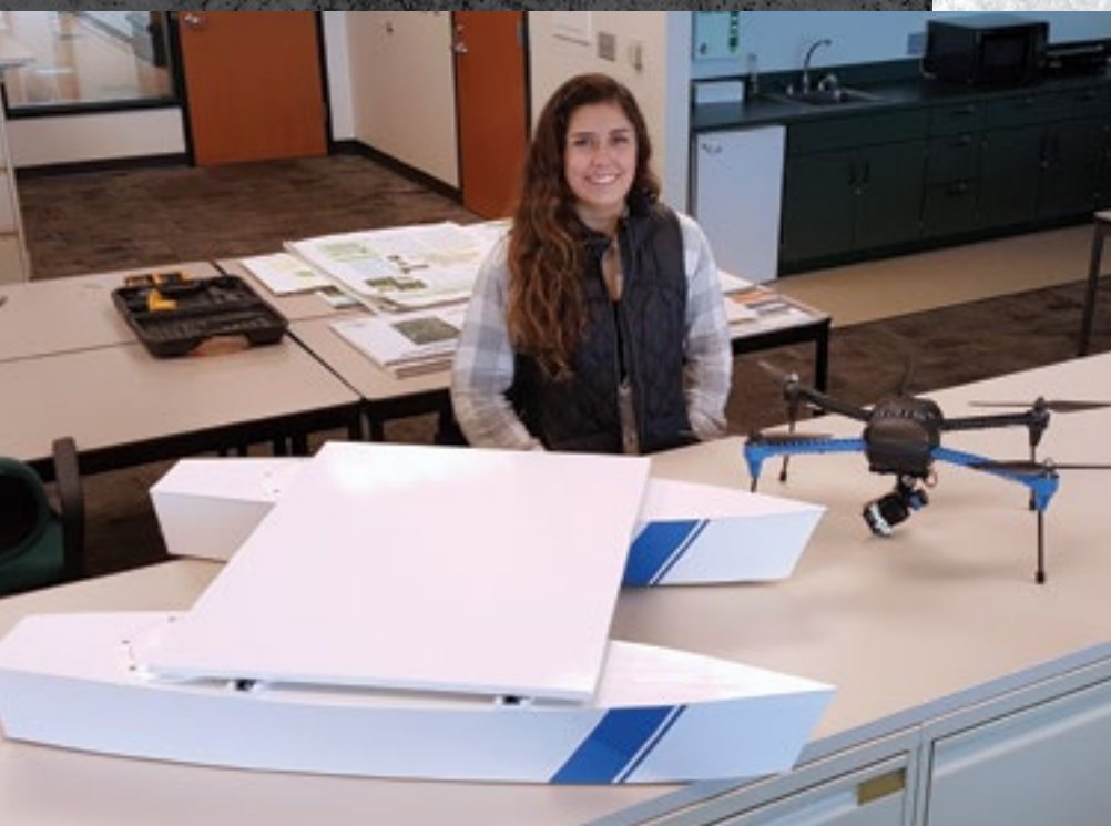
Gabrielle Thelen with AWRI's BoatBot and commercially available quadcopter to be used together to test their wireless tether capability for water quality research.
