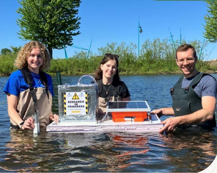
Ashtyn Gluck (left), Jillian Greene (center), and Dr. Sean Woznicki (right) deploy a DIY GHG chamber at Heritage Landing on Muskegon Lake. Photo credit: Bopi Biddanda.
