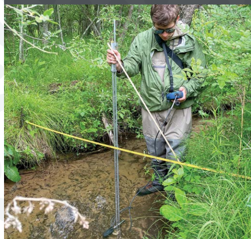
Technician Grayson Kosak measures water velocity in Swinton Creek, a tributary of the White River. Photo Credit: Carl Ruetz.
