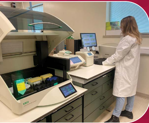
Research assistant Alexis Porter conducts ddPCR testing of wastewater samples. Photo Credit: Brian Scull.
