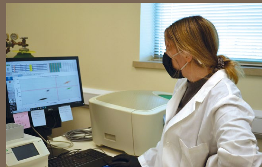
Research assistant Alexis Porter conducts ddPCR testing on wastewater samples for COVID-19 delta variant.
