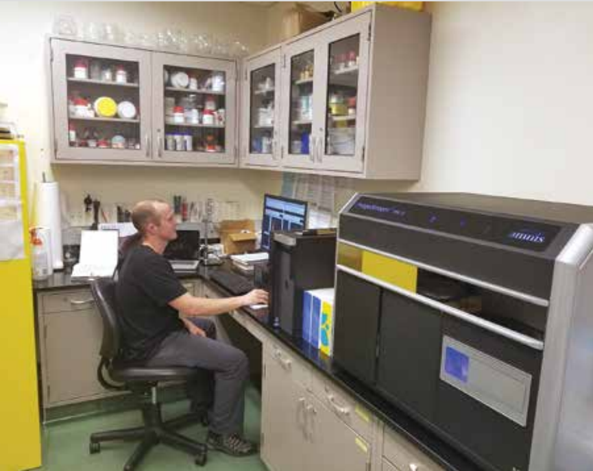
GVSU undergraduate intern Darrick Gates developing faster methods to study Escherichia coli ( E. coli ) in food contamination using state-of-the-art imaging flow cytometry. Photo Credit: Nate Hoekstra
