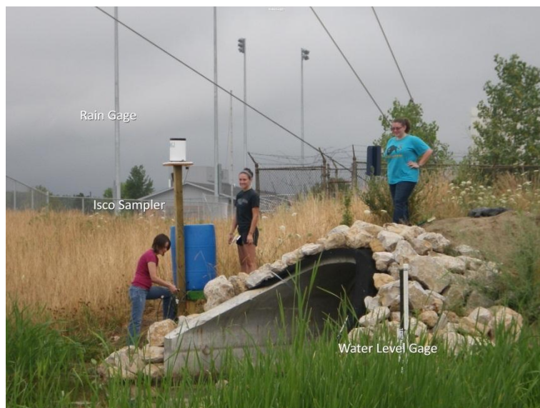
Figure 3. Wetland Sample Site S1 (pond #1). The Isco sampler is in the blue barrel and the rain gage trigger is on the post.
