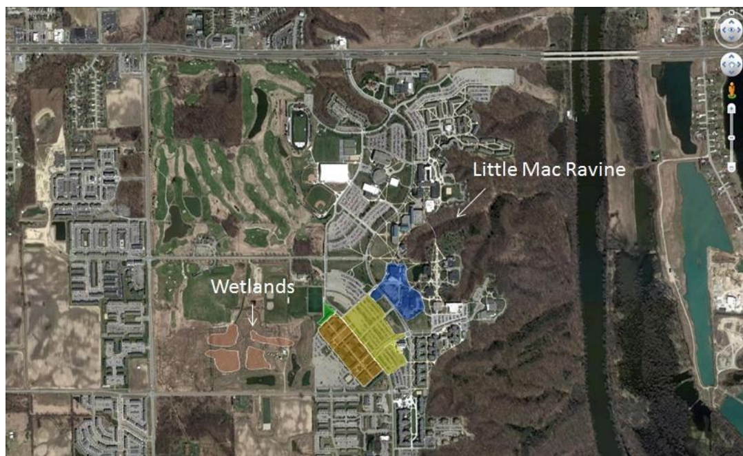
Figure 2. Little Mac Ravine sampling and monitoring location. Colored area is the area of parking lots diverted into the pond complex show in brown.
