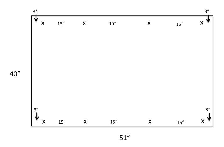
All measurements are the to center of the holes.
