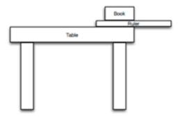
The students should explore what it takes to make different sounds. The <u>length</u> of the ruler hanging off the edge determines the <u>pitch</u> of the note produced. The <u>force</u> of the plucking action determines the <u>loudness</u> of the note produced.
