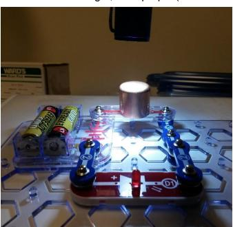
If the red diode does not light, it is opaque (as shown below).
