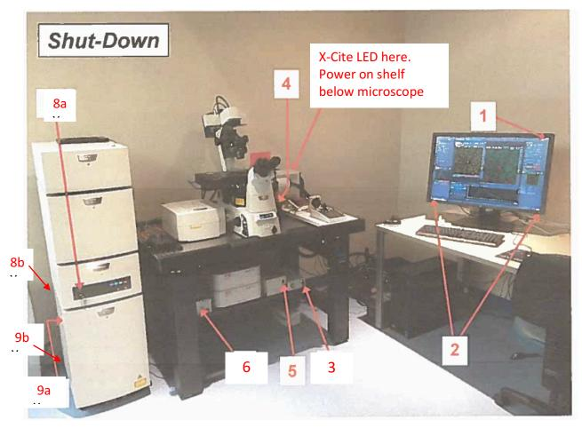
For Shut-Down of the software and hardware work backward from the start up steps. Before starting these steps, make sure to a) lower the objective to the lowest position, b) remove slide and clean oil from objective, c) turn objective to open position.
