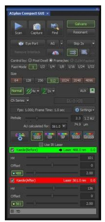
3. In the A1 Stimulation control box, press the 405 button to use that line for photoactivation. The optimal laser power for photoactivation will require some experimenting. Too little power will have no effect (red & green signals won't change) and too much power will cause bleaching rather than activation (red & green signals both decrease). In this example, I used 30% for a single 1fps pass.
