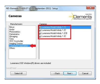
9) In the 'Cameras' dialog, select 'Lumenera' under 'Manufacturers' and then choose all camera models. This will insure all necessary files will be installed.
