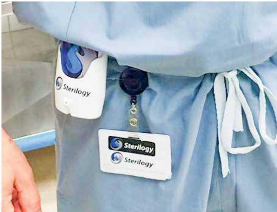
This hand hygiene system alerts user and records information to aid in organization compliance rates.
