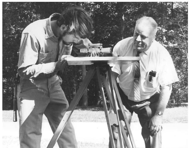
Johnny Lucke and Dick Page doing plane table and alidade mapping (source Bill Neal?)
