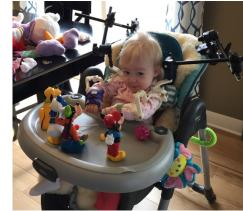
interaction with a Type I/II SMA patient to provide the necessary degrees of freedom, range of motion, and loading. The design and FEA analysis employed SolidWorks<sup>TM</sup>. After development, several prototypes and the final product were rapid prototyped using a Dimension 1200es.
