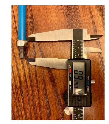
Thread length is verified by measuring the distance from the end of the rod to the end of a nut that is fully threaded on the rod. The thread length has a tolerance of 1/16"
