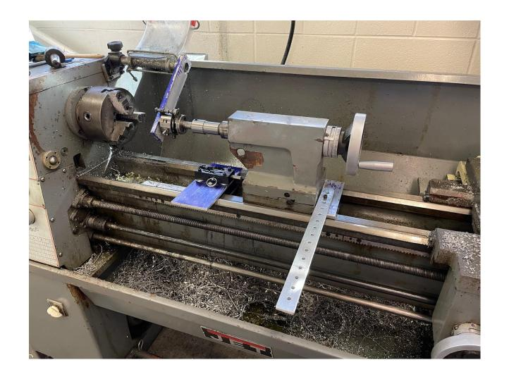
Prototyping involved creating a manual version of our final design. This allowed for testing thread quality, the speed at which the spindle could be run at, and the forces required to start and stop threading.
