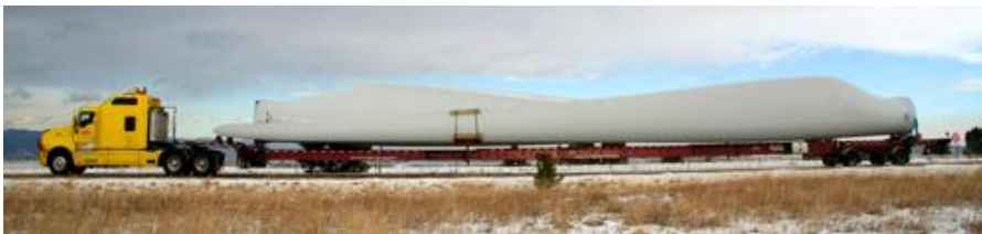
Figure 4a. Transporting a turbine blade of 1.5 MW test turbine, which when complete have a rotor diameter of 250 feet. (Colorado, 2008)
