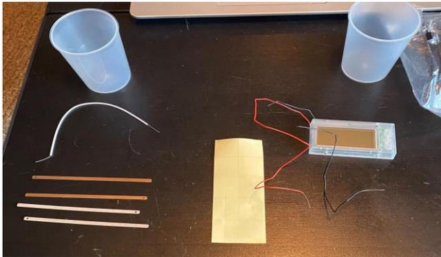
2. Begin activity by threading one side of the loose wire through the hole of one of the brown plates then wrap and spin it tightly to where it holds to the plate
