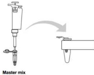
5. Remove your PCR tube from the capless micro test tube and place the tube in the thermal cycler.
