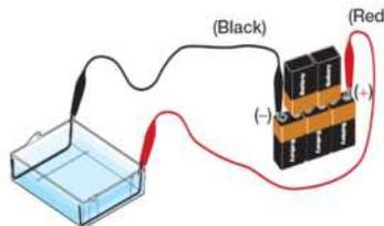
12. Allow your gel to run for 20 min. Disconnect the red and black alligator clips from the battery tower.
