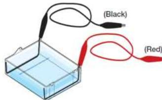
11. When you are ready to begin your electrophoresis run, attach the free black alligator clip on your lead to the (-) terminal of your battery tower and the free red alligator clip on your lead to the (+) of your battery tower. You should notice bubbles coming off of the paper clip electrodes if the circuit is complete.
