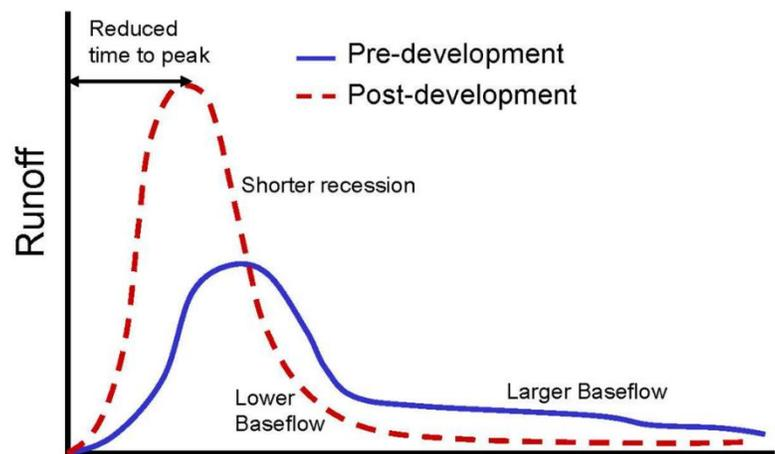
Figure 1. Hydrograph illustrating the difference in stream flow in an urban, developed setting and pre-urban development condition. Source: Liu, J.; Sample, D.J.; Bell, C.; and Guan, Y. (2014) Review and Research Needs of Bioretention Used for the Treatment of Urban Stormwater. *Water* 6(4), 1069-1099. Available online at: <http://www.mdpi.com/2073-4441/6/4/1069/html>
