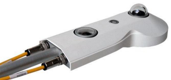
Measures incoming and reflected short wave (380-2500nm) and long wave (4500-42,000nm) radiation
