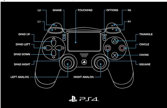
To use the PS4, connect the controller via the following:
