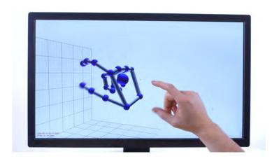
The sensor connects to a computer using an USB port. The computer will gather raw data from the sensor and the software system embedded in the computer will decide based on the gesture type which command it should send to the quadcopter (Figure 8).
