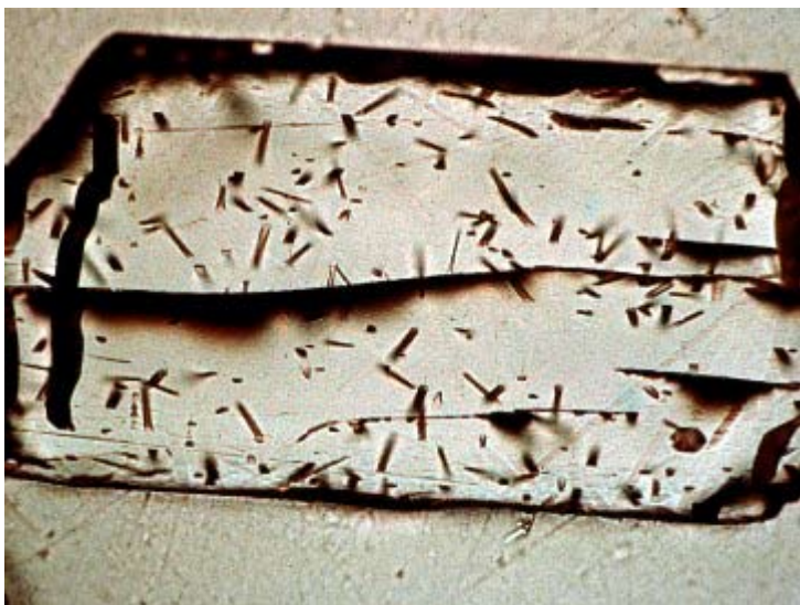
Figure 2a. Etched spontaneous fission tracks within an apatite crystal. http://www.geotrack.com.au/afta-overview.htm
