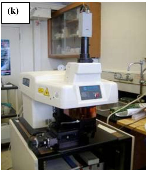
Figures 3g-l. (g) After centrifuging and rinsing, air drying the remaining sediment in a small Petri dish. (h) Frantz Isodynamic magnetic separator. (i) Grain mounts that used epoxy-only. (j) High power microscope, coordinate system digitizer, and computer. (k) LA-ICP-MS. (l) Californium-252 source.
