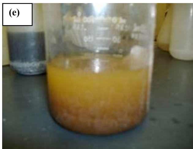
Figures 3a-f. Mineral separation procedures. (a) Jaw crusher used to crush samples. (b) 300 micron sieve cloth. (c) Sieved material \leq 300 microns. (d) Washing the fine-grain mud and clay particles. (e) Heavy mineral separation using lithium metatungstate (LMT). (f) Centrifuge.
